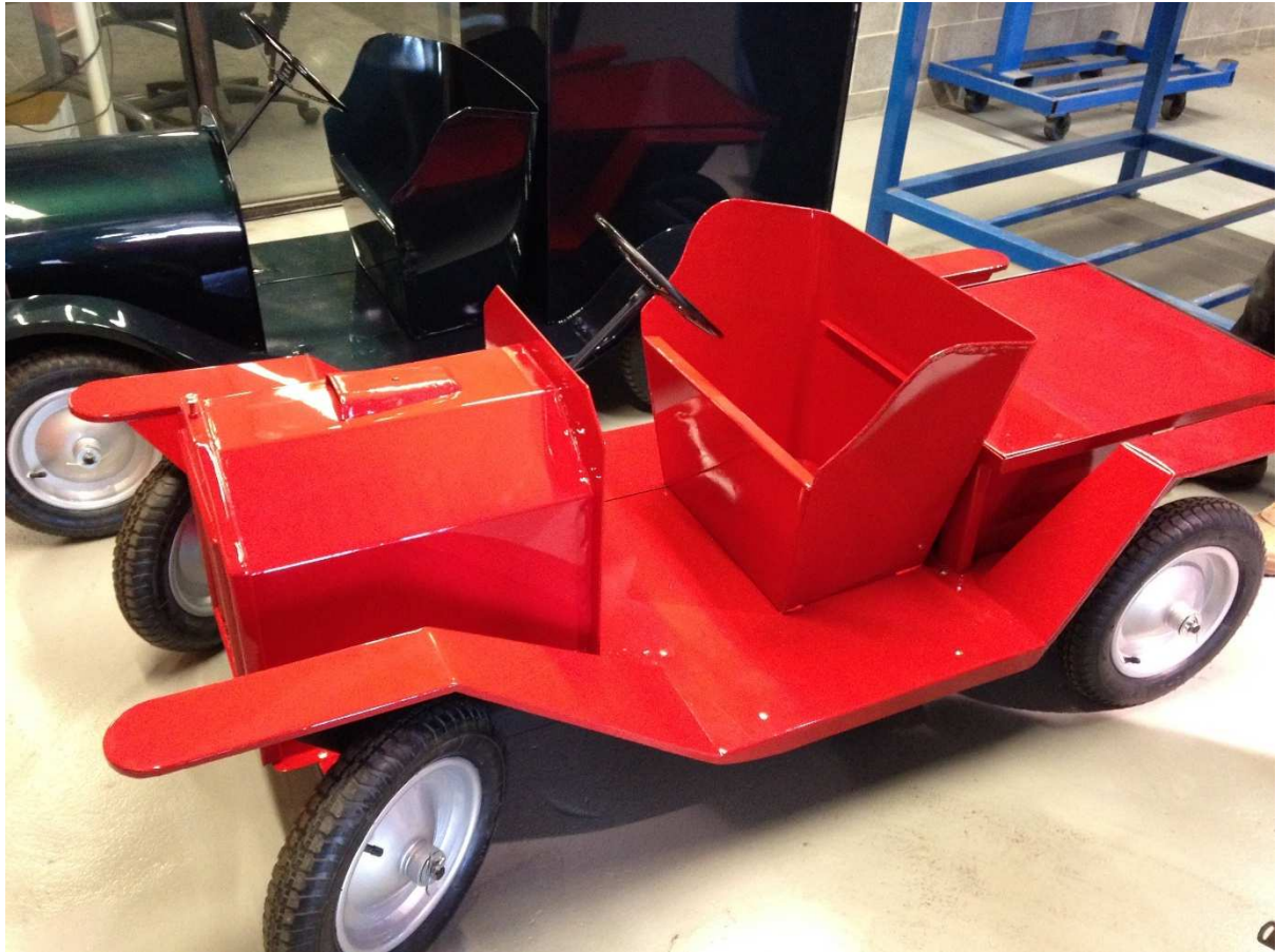
Fig 1: An example of a product produced in a work for the Dole activity. This is a pushcar produced by students using welding and fabrication skills.
